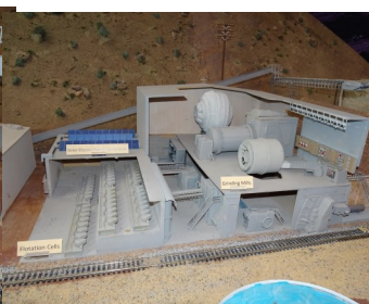
Grinding Mills & Flotation
