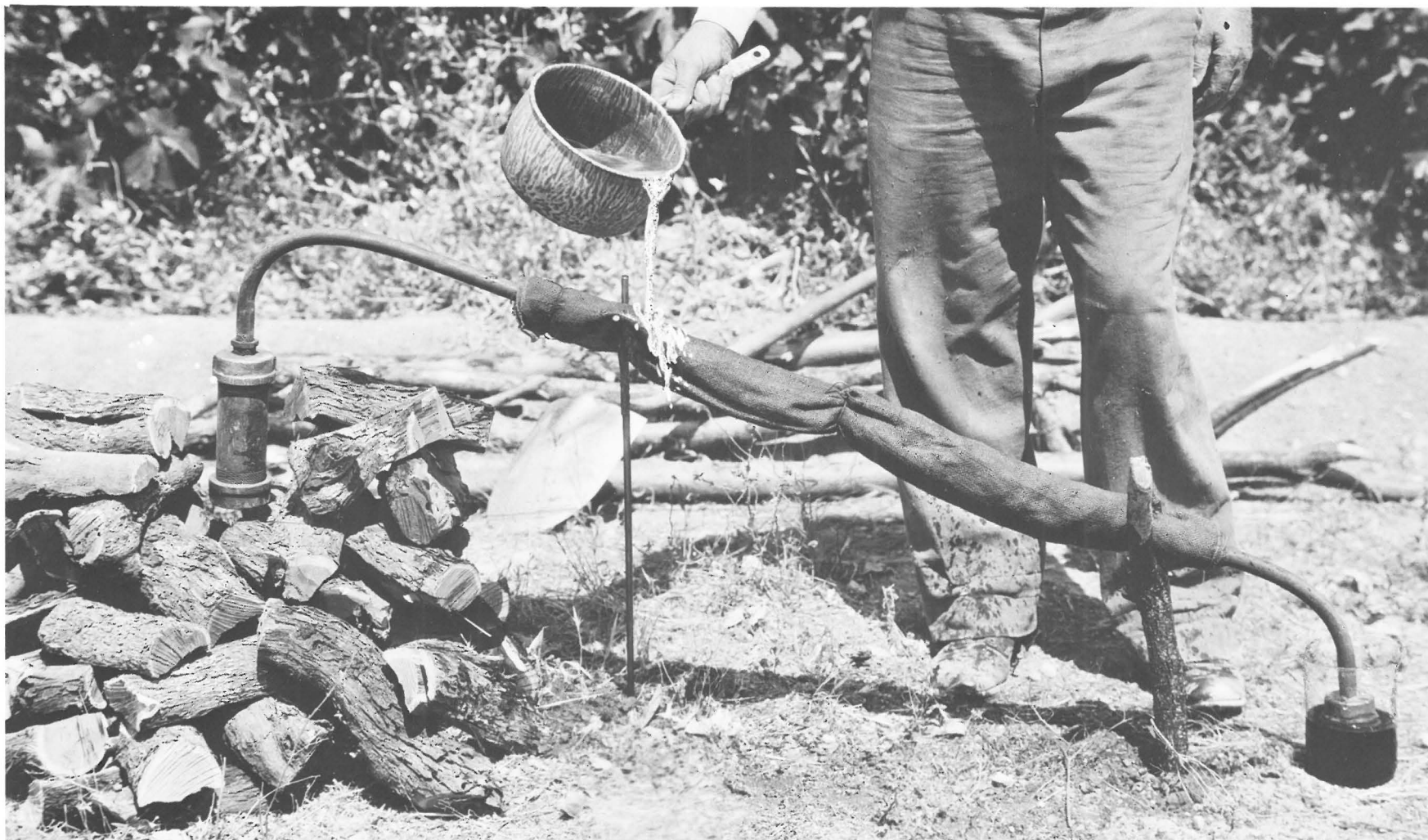
Homemade retort used to separate mercury from gold amalgam. Mercury vapor is condensed to liquid and recovered in beaker containing water. Courtesy of the Arizona Geological Survey.
